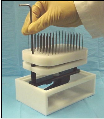
Figure 6: Transfer device placed in wash stand for removal of screws
