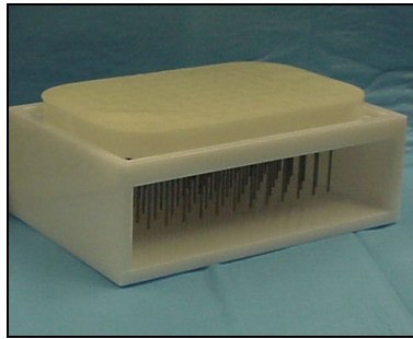
Figure 15: Transfer device with plunger plate and seal plate removed and gasket exposed for inspection
