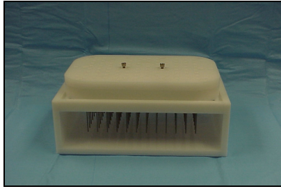
Figure 14: Needle plate in wash stand with all but 2 screws removed
