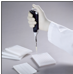
Figure 1: Using Well Identification Templates to Aspirate a Sample from a 384-Well PCR Tray
